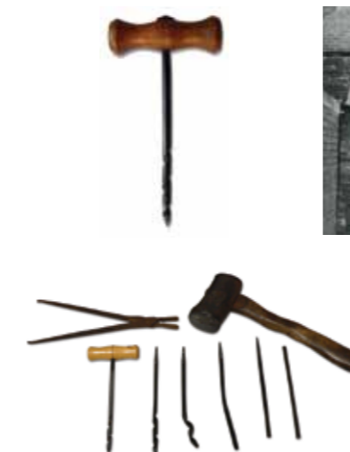
Opposite: gimlet making tools and stages in the production of a gimlet
